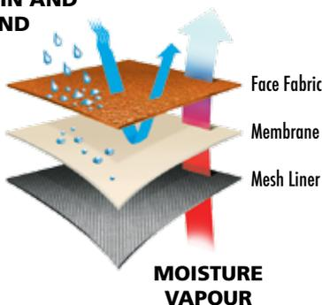
*The PTFE membrane is totally waterproof. Yet it allows moisture vapour to pass through, thus keeping you dry from both the inside and outside elements.*
